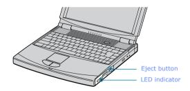
Do not push the eject button when the LED indicator is turned on. Otherwise, data may be lost.
